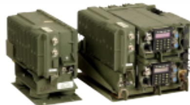
AN/VRC-92 Vehicular 50W dual long-range (retransmit)– plus 2nd power amp and retrans cable
