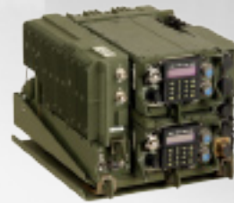
AN/VRC-89 Vehicular 50W long-range/short-range
